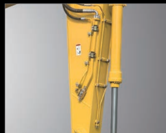
Quick Coupler Piping*
