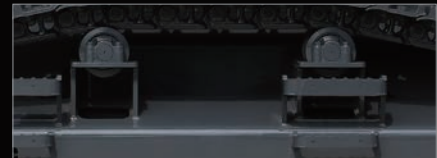
2 Large, double-support, outer flanged upper rollers
