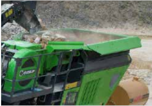
HOPPER BOLT ON PROTECTOR PLATES
