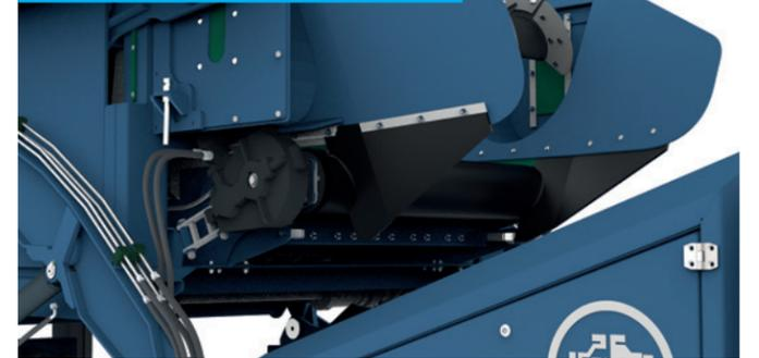
By means of carbide scrapers, the conveyor belts of the mobile 3D COMBI screen is cleaned of sticky and/or strongly adhering materials, such as clay, plaster, cement...
