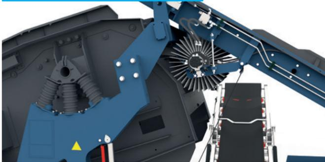
Using the cleaning brush for the infeed belt means that less material remains stuck on the belt, which also results in less fine-grained leakage material underneath the machine.
