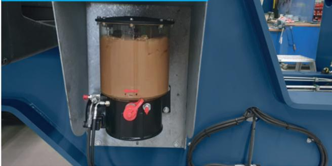
The automatic central lubrication system ensures the reliable operational readiness of the 3D COMBI screen by constant renewal of the lubricating film.
