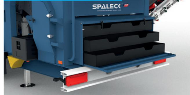
A screening mats box is optionally available for the safe and easy storage of the different screening mats of the 3D COMBI screen.
