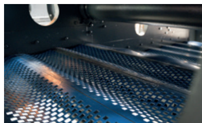
Lower deck of the Flip-Flow screen
