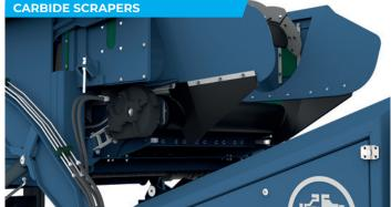
By means of carbide scrapers, the conveyor belts of the mobile 3D COMBI screen is cleaned of sticky and/or strongly adhering materials, such as clay, plaster, cement...
