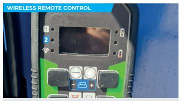
To significantly reduce the time and personnel required, the remote control allows comfortable control of the mobile 3D COMBI screen even from the wheel loader.
