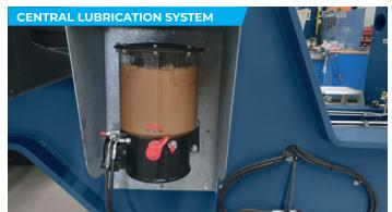
The automatic central lubrication system ensures the reliable operational readiness of the 3D COMBI screen by constant renewal of the lubricating film.
