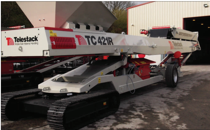
1.8 metre (6ft) crawler track mounted unit
