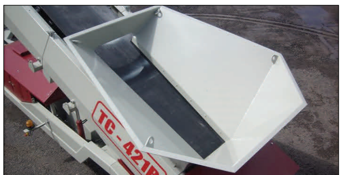
Hexagonal feed-boot - 2.39m x 2.22m (7'9" x 7'3")
