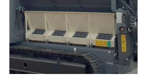
Full chamber access for servicing and breaker bar replacement
