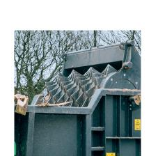
Intelligent feed wheel with lift and downward assist
