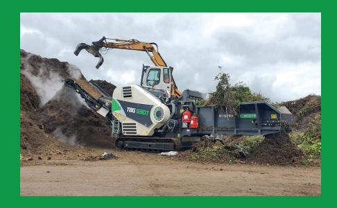
With a rapid set up time the TBG 530T is ready to work in a matter of minutes with no tooling required. The open fronted feeder enables the TBG 530T to be fed quickly and easily from the rear. The intelligently controlled feed system, comprising of heavy duty drag chains and aggressive feed wheel with unique lift/downward assist, ensure optimum material flow resulting in class leading performance.
