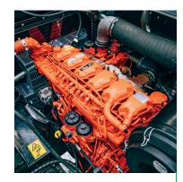
368kW (493HP) Scania DC 13 Stage V Unrivalled service access Direct drive rotor for efficient shredding
