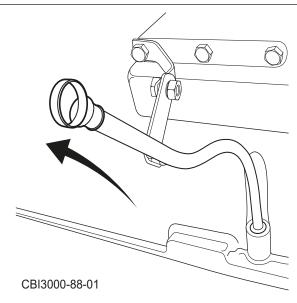
Figure 6.26 - Remove Engine Oil Dipstick
