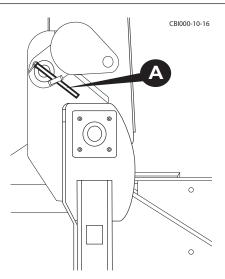
Figure 5.77 - Install Locking Pin (5800 Series)
