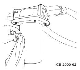
Figure 6.56 - Clean Filter Housing
