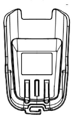
Figure 5.42 - Remote Control Charging Cradle
