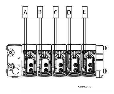
Figure 2.11 - Manual Control Valves
