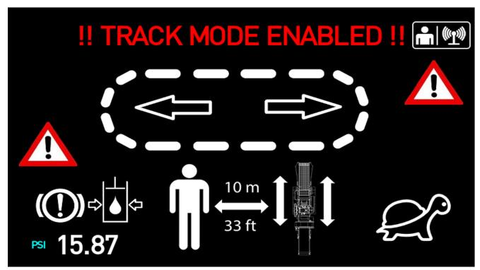
Figure 5.38 - Track Mode Enabled - Indicates Track Mode is enabled.
