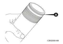
Figure 6.54 - Inspect Filter Housing Seal
