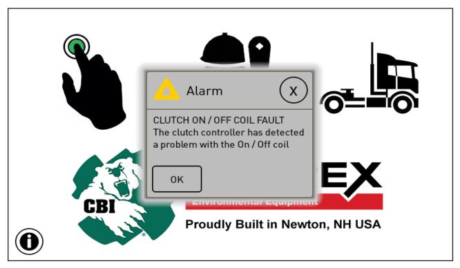
Figure 5.40 - An example of PT Tech Diagnostic Message, Pressing the X will close the Diagnostic Message.
