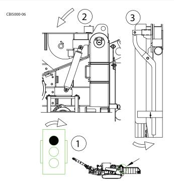
Figure 5.78 - Remove Locking Pin (6400/6800 Series)
