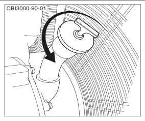
Figure 6.29 - Remove Fill Plug
