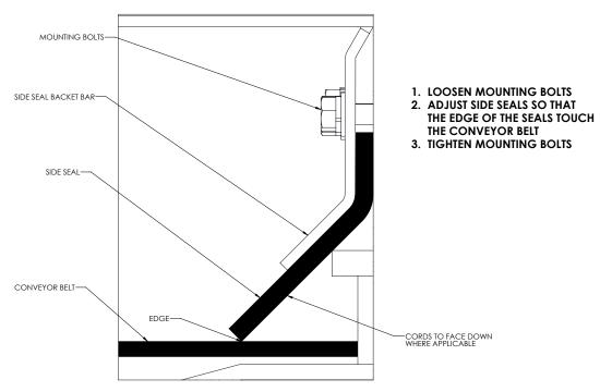
Figure 6.21 - Side Seal Adjustment Diagram
