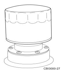
Figure 6.49 - Remove/Inspect Breather Element
