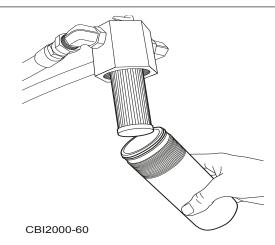
Figure 6.57 - Remove Bowl from Filter Housing
