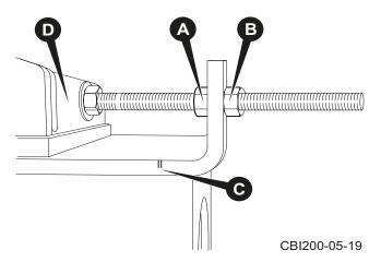
Figure 6.3 - Adjust Take-Up Rod Nuts
