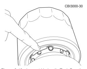
Figure 6.48 - Inspect Hydraulic Tank Breather
