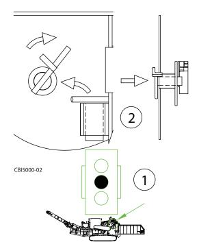
Figure 5.74 - Top Roll Safety Lock Pin (6400/6800 Series)
