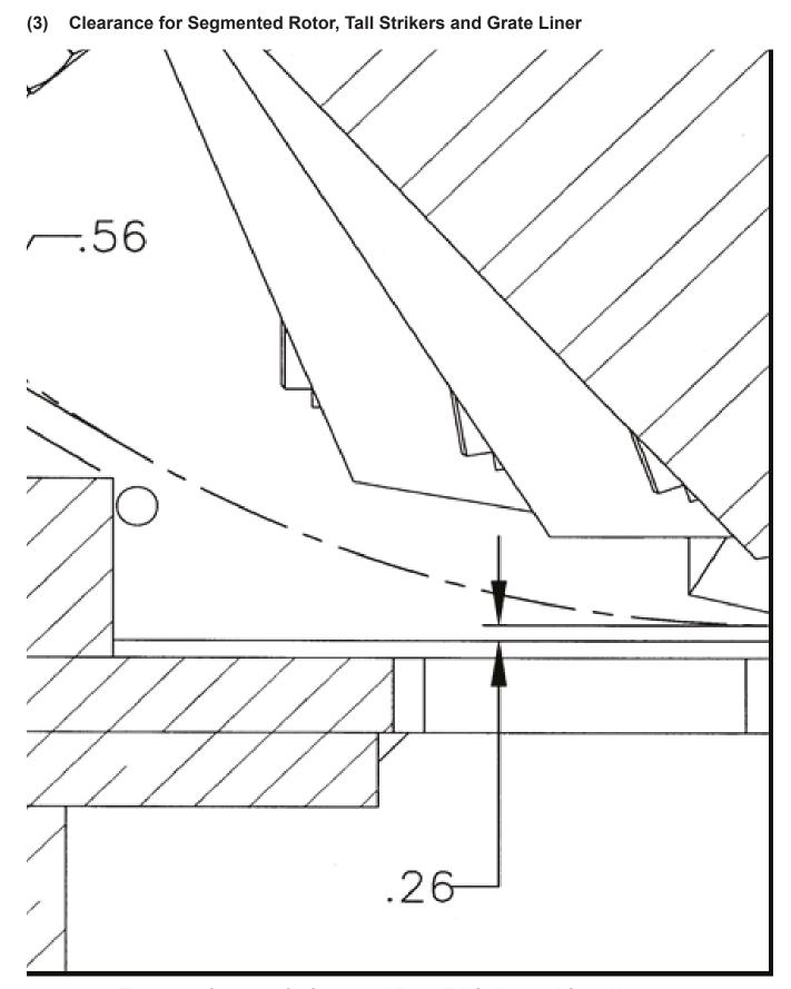
Figure 6.5 - Clearance for Segmented Rotor, Tall Strikers and Grate Liner
