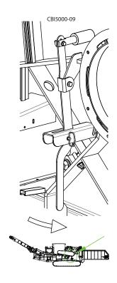
Figure 5.82 - Remove Grate Retention Pin (6400/6800 Series)
