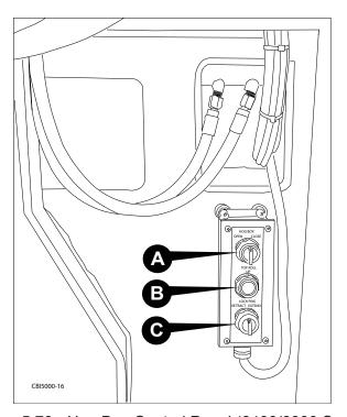
Figure 5.70 - Hog Box Control Panel (6400/6800 Series)
