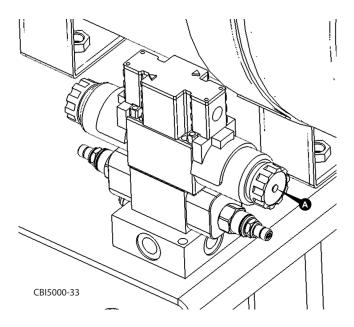
Figure 2.9 - Belt Engage Valve Manual Override
