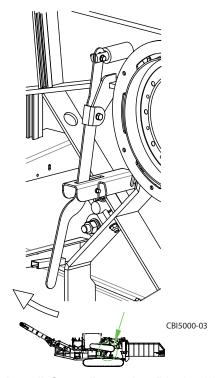
Figure 5.72 - Install Grate Retention Pin (6400/6800 Series)
