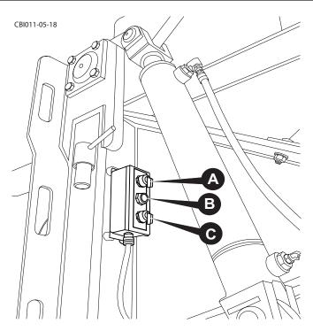
Figure 5.71 - Hog Box Control Panel (5800 Series)
