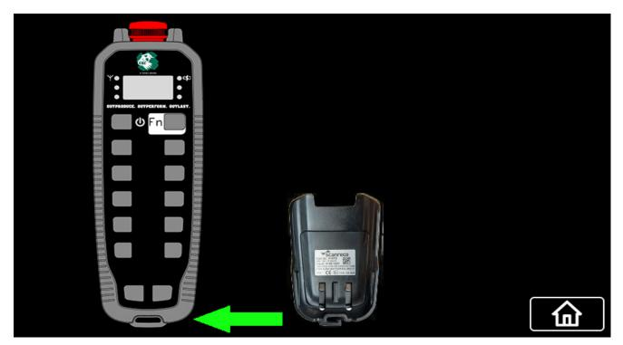
Figure 5.11 - Plug in Remote Control
