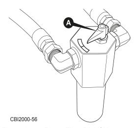
Figure 6.55 - Reset Filter Dial if Necessary
