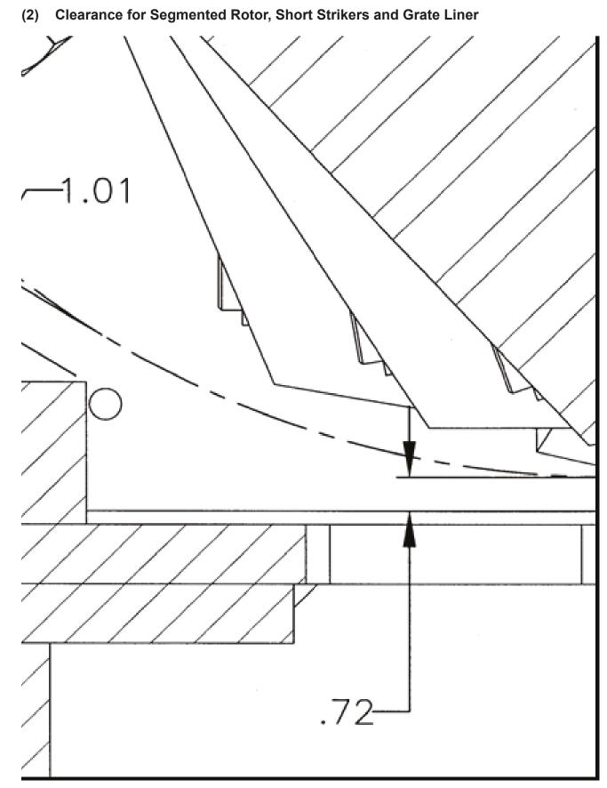
Figure 6.4 - Clearance for Segmented Rotor, Short Strikers and Grate Liner
