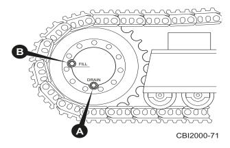
Figure 6.34 - Track Drain and Fill Plugs
