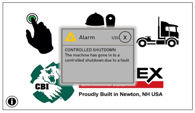
Figure 5.36 - An example of a CBI Diagnostic Message, Pressing the X will close it.
