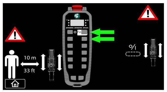
Figure 5.7 - Enable Track Mode on the Remote
