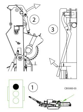
Figure 5.76 - Install Locking Pin (6400/6800 Series)
