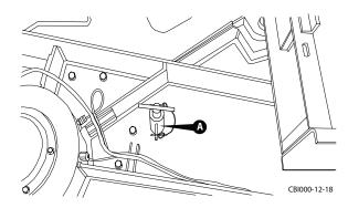
Figure 5.73 - Install Grate Retention Pin (5800 Series)
