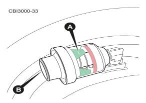
Figure 6.45 - Inspect Air Filter Indicator
