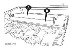
Figure 6.18 - Remove Grate Liner
