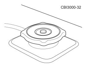
Figure 6.38 - Engine Coolant Fill Cap
