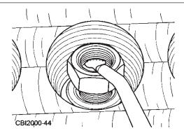
Figure 6.10 - Lubricate stud threads
