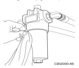
Figure 6.51 - Clean Filter Housing
