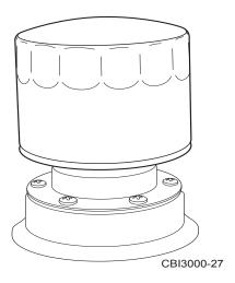
Figure 6.47 - Inspect Hydraulic Tank Breather
