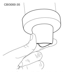
Figure 6.46 - Squeeze Air Filter Unloader Valve
