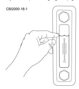
Figure 6.23 - Check Hydraulic Oil Level Site Gauge
