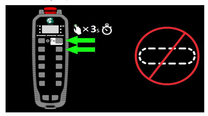
Figure 5.9 - Disable Track Mode on the Remote
