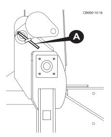
Figure 5.79 - Remove Locking Pin (5800 Series)
