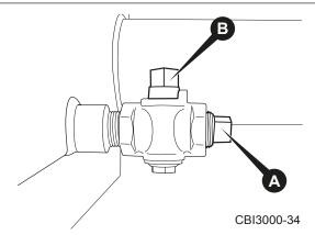
Figure 6.39 - Engine Coolant Drain Valve
