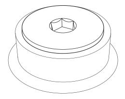
Figure 6.25 - Remove Fill Plug from Hydraulic Oil Tank
