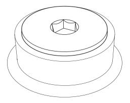
Figure 6.24 - Remove Fill Plug from Hydraulic Oil Tank
