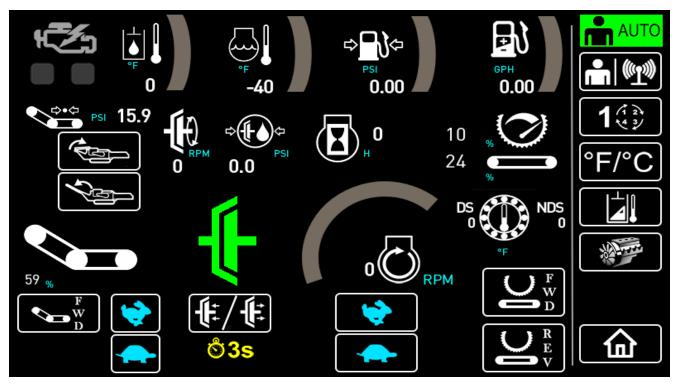
Figure 5.16 - Basic Run Menu (Clutch-Equipped Machine)
