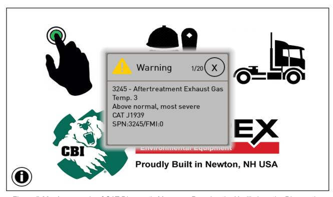
Figure 5.39 - An example of CAT Diagnostic Message, Pressing the X will close the Diagnostic Message.
