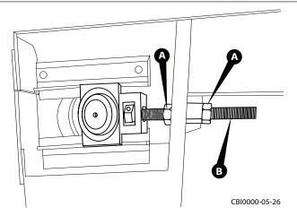
Figure 6.20 - Loosen Adjustment Rod Lock Nuts
