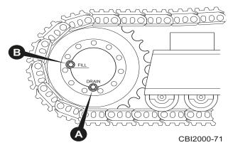
Figure 6.35 - Track Drain and Fill Plugs
