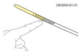
Figure 6.27 - Inspect Oil Level on Dipstick
