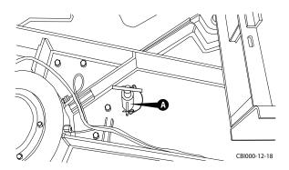
Figure 5.83 - Retention Pin
