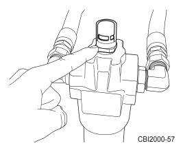
Figure 6.50 - Inspect Filter Indicator
