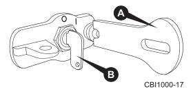
Figure 2.6 - Engine Battery Disconnect Switch Door and Key
