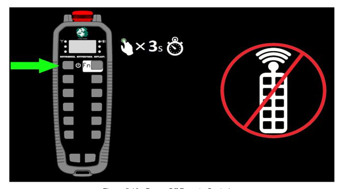
Figure 5.10 - Power Off Remote Control
