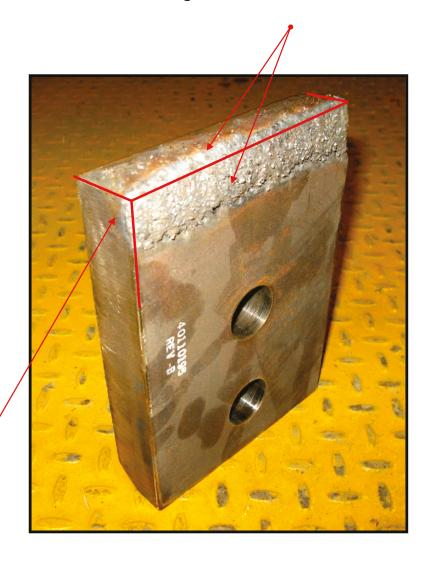
Rebuild striker to original profile by using 3/16" buildup rod, Terex part number 80013148 when wear exceeds 1/4". Do not use hard face rod as buildup.
