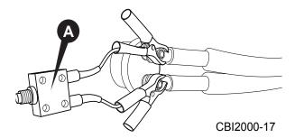
Figure 6.62 - Mount Safety Breaker Across Terminals
