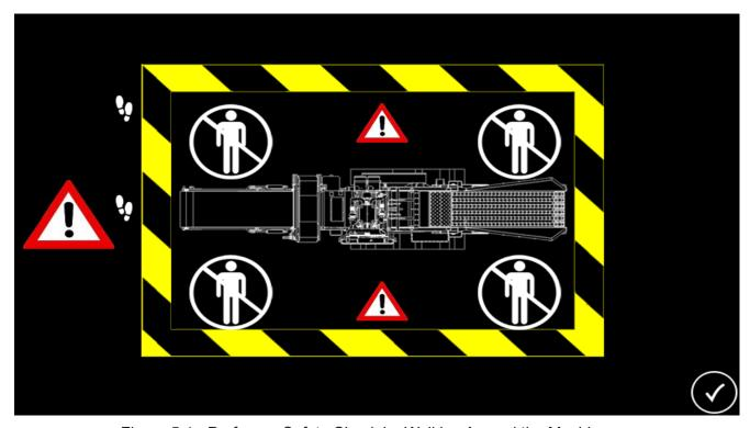
Figure 5.4 - Perform a Safety Check by Walking Around the Machine
