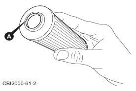
Figure 6.58 - Install Filter Element
