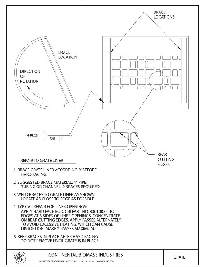
Figure 6.19 - Grate Hard Surfacing Drawing
