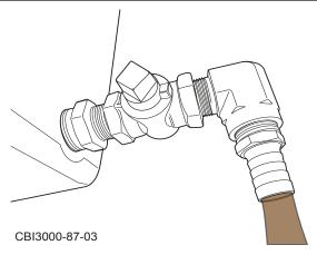
Figure 6.32 - Drain Engine Oil
