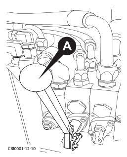
Figure 5.85 - Manual Control Valves (5400 Series)
