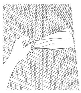
Figure 6.43 - Verify Fan Direction
