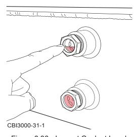
Figure 6.36 - Inspect Coolant Level
