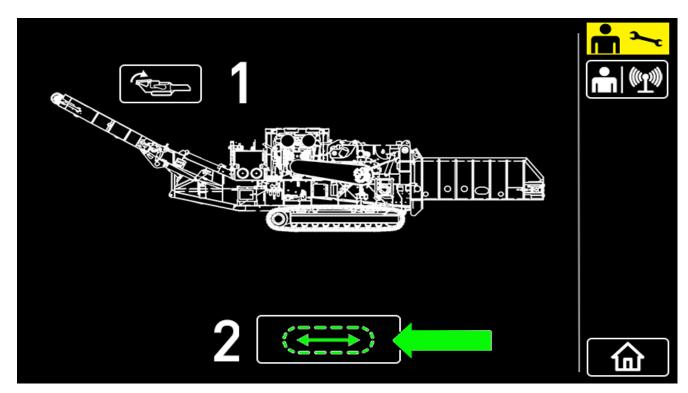
Figure 5.3 - Enable Track Mode
